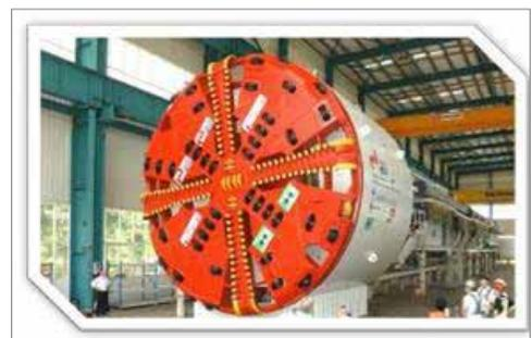
**Figure E-8. Typical Pressurized-Face TBM**
