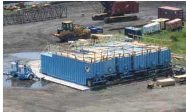
**Figure E-14. Typical Slurry Mixing Plant**
