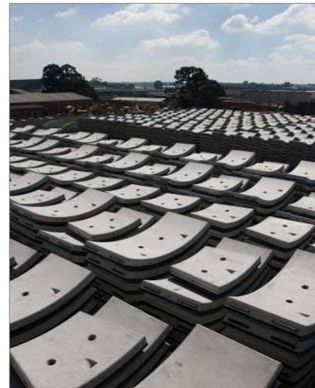
**Figure E-17. Precast Concrete Segments Storage**
